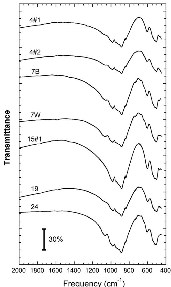
Fig. 5. The 2000–450  $\text{cm}^{-1}$  (5.0–22.2  $\mu\text{m}$ ) infrared transmission spectra of seven samples dominated by olivine taken from five stones of the Almahata Sitta meteorite.
