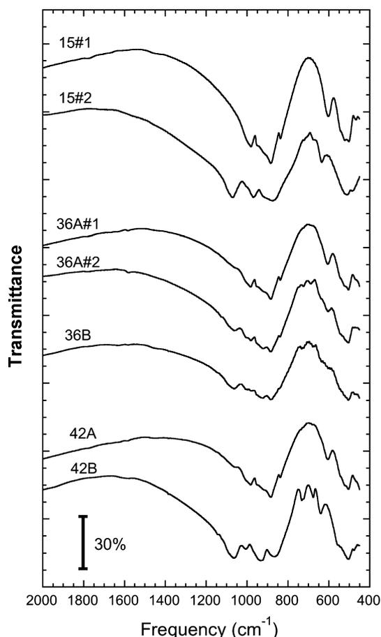
Fig. 11. The 2000–450  $\text{cm}^{-1}$  (5.0–22.2  $\mu\text{m}$ ) infrared transmission spectra of seven samples taken from three stones of the Almahata Sitta meteorite. In many cases, the spectra of multiple samples from the same stone show very similar spectra, but spectra from these three stones show some of the most dramatic variations.
