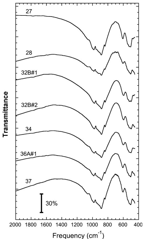
Fig. 6. The 2000–450  $\text{cm}^{-1}$  (5.0–22.2  $\mu\text{m}$ ) infrared transmission spectra of seven samples dominated by olivine taken from six stones of the Almahata Sitta meteorite. The spectrum of sample 32B#2 was used as the olivine spectral endmember for the determination of olivine-to-pyroxene ratios in all the samples.
