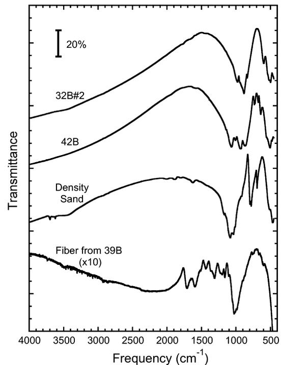
Fig. 3. The 4000–450  $\text{cm}^{-1}$  (2.5–22.2  $\mu\text{m}$ ) infrared transmission spectra of Almahata Sitta endmember samples 32B#2 (olivine) and 42B (pyroxene), a sample of the contaminant “sand” used to make previous density measurements of the meteorite, and contaminant fibers found in sample container 39B for stone #39.
