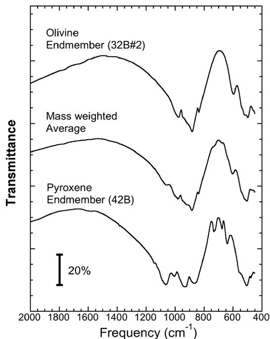
Fig. 10. The 2000–450  $\text{cm}^{-1}$  (5.0–22.2  $\mu\text{m}$ ) infrared transmission spectra of the mass weighted average spectrum of all the infrared spectra taken from Almahata Sitta, except stone 25, compared to the spectra of the olivine and pyroxene spectral endmembers (32B#2 and 42B, respectively). The averaged spectrum is consistent with an olivine-to-pyroxene mixture of 74:26.
