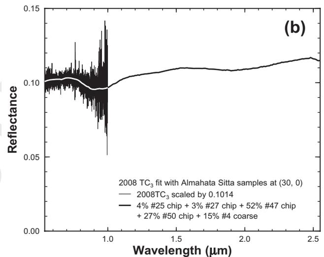
Fig. 7. Linear least-square fits of the observed reflectance spectrum of asteroid 2008 TC<sub>3</sub> (courtesy of Alan Fitzsimmons) with the VNIR spectra of two different sets of Almahata Sitta meteorite samples: a) chip samples measured at 19° incidence and 0° emergence angles (Fig. 2a), and b) chip and powder samples measured at the standard viewing geometry (Figs. 2 and 5). The asteroid reflectance spectrum was scaled up or down for the best match with the combined laboratory spectra.
