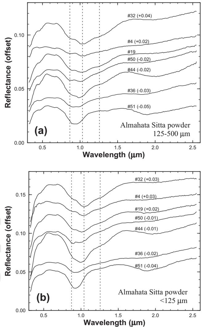
Fig. 5. Bidirectional VNIR reflectance spectra of (a) coarse powder samples (125–500 μm) and (b) fine powder samples (<125 μm) of Almahata Sitta meteorite measured at the standard viewing geometry. Reflectance values are offset by the amounts indicated in parentheses after the stone numbers for clarify. Vertical broken lines indicate approximate wavelength positions of three absorption bands of olivine.
