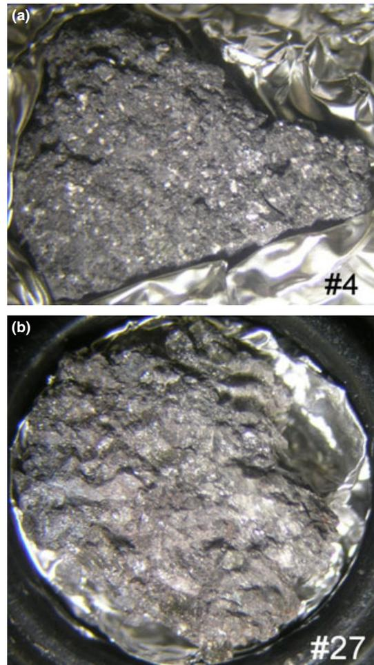
Fig. 1. Photos of chip samples of Almahata Sitta meteorite stones #4 and #27, embedded in aluminum foil for reflectance spectral measurements. The longest dimensions of the chips are about 1.4 and 1.0 cm, respectively.
