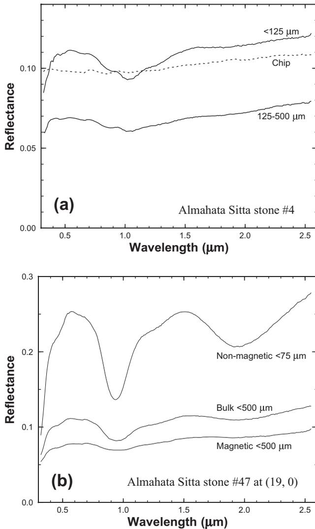
Fig. 4. Comparison of VNIR reflectance spectra of some samples of Almahata Sitta meteorite. a) Chip and powder samples of stone #4 measured at the standard viewing geometry. b) Bulk powder sample and magnetic and nonmagnetic portions of stone #47 measured at 19° incidence and 0° emergence angles.
