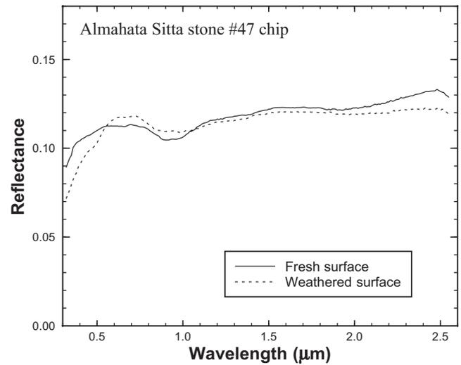
Fig. 3. Fresh and weathered surfaces of stone #47 chip measured at the standard viewing geometry.
