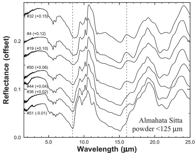
Fig. 6. Off-axis biconical Fourier-transform infrared (FT-IR) reflectance spectra of fine power samples (<125  $\mu\text{m}$ ) of Almahata Sitta meteorite. Reflectance values are offset by the amounts indicated in the parentheses for clarity. Indicated with broken lines are the Christiansen feature around 8.4  $\mu\text{m}$  and another feature around 16  $\mu\text{m}$  which may be indicative of compositional change.
