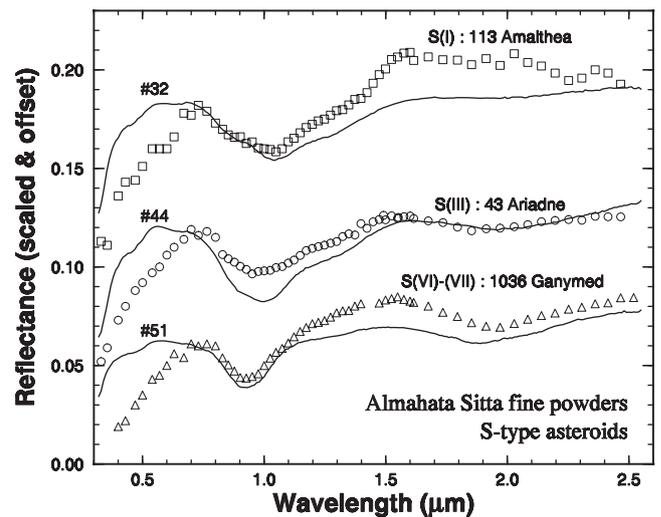
Fig. 8. Comparison of the VNR spectra of fine powder samples of some Almahata Sitta meteorite stones and S-type asteroids (Chapman and Gaffey 1979; Bell et al. 1988).
