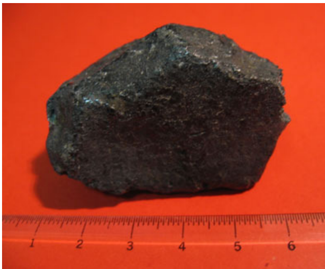
Fig. 1. Fragment #15 of Almahata Sitta, weighing 75 g. The scale is in cm. The shape of this fragment is important for determination of the gamma acquisition efficiency, for which its mold labeled with known radioisotopes was made.
